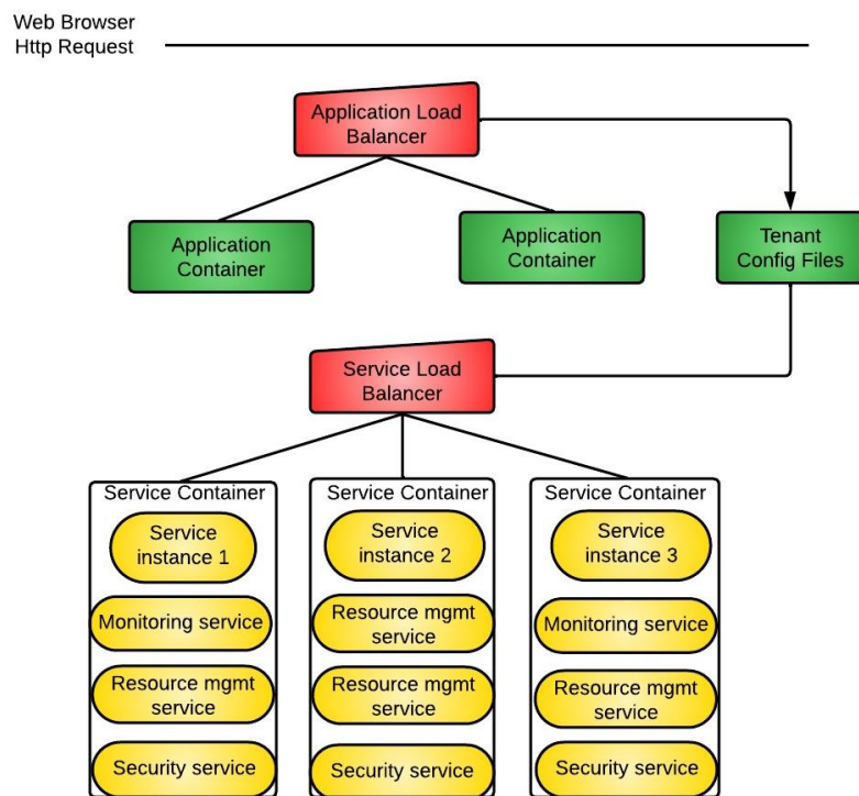
Figure 1: Single Application Instance Multiple Service Instances
